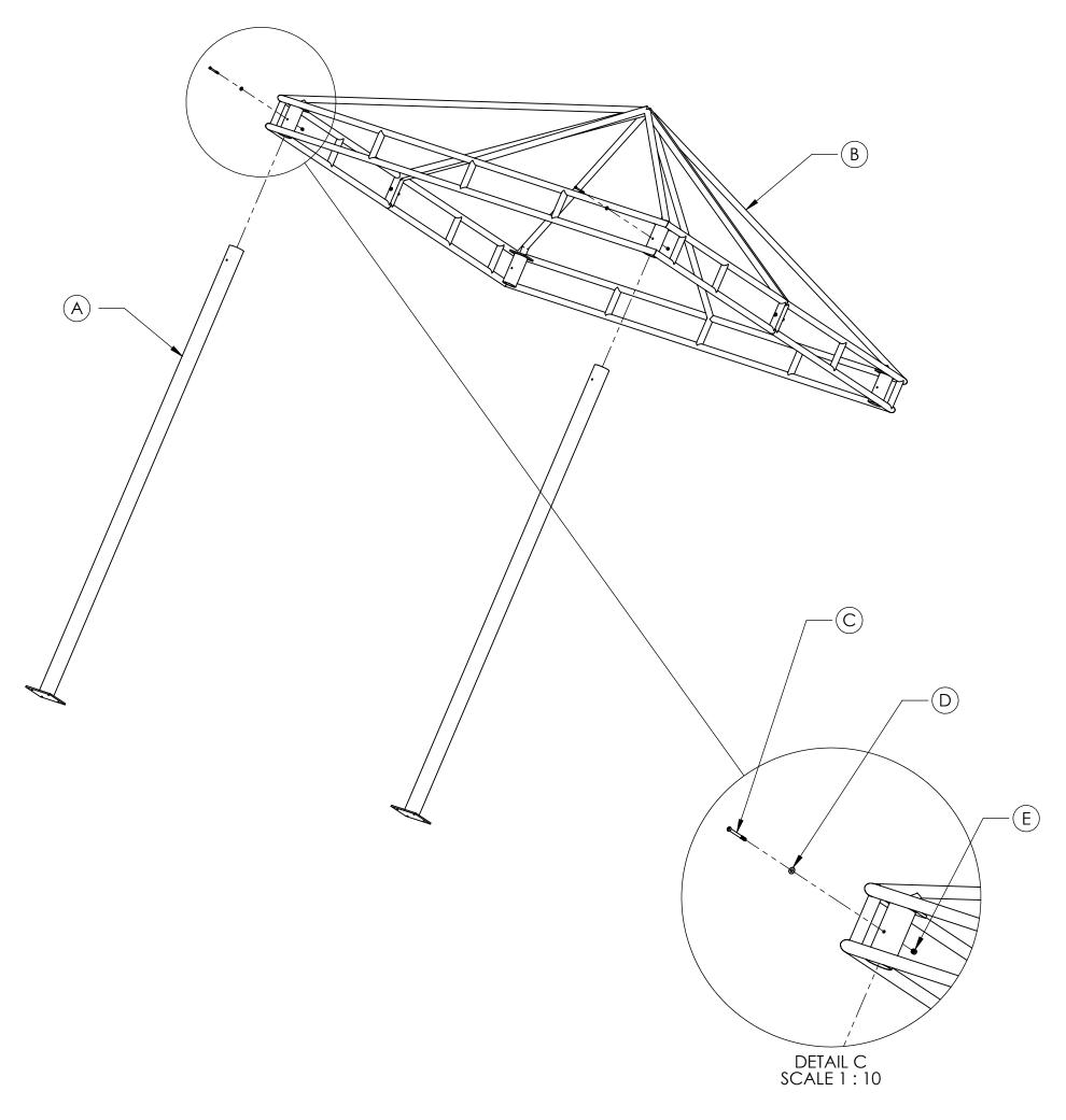
NOTE: - LINE UP BOTH LEGS BY LINING UP THE HOLES AND INSERTING THE SCREWS. (AS SHOWN)
